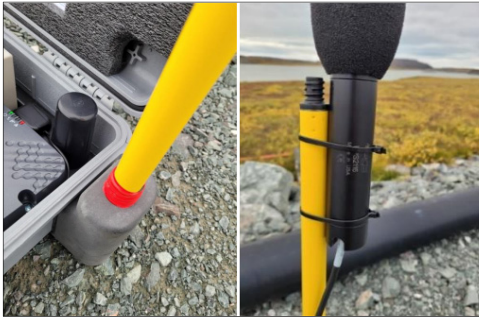
Photo 1 Microphone affixed to vertical pole.
