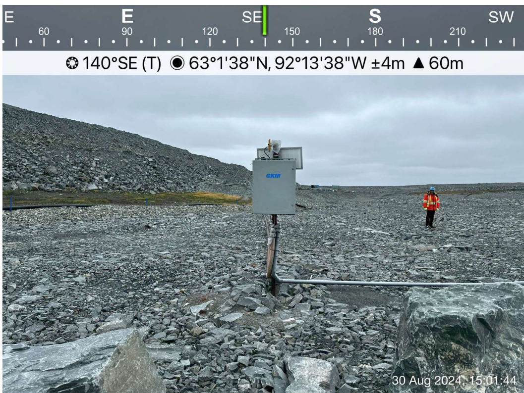
CP4 Thermal Berm Photo 4: CP4 Thermal Berm - GTC data collection system. Facing southeast.
