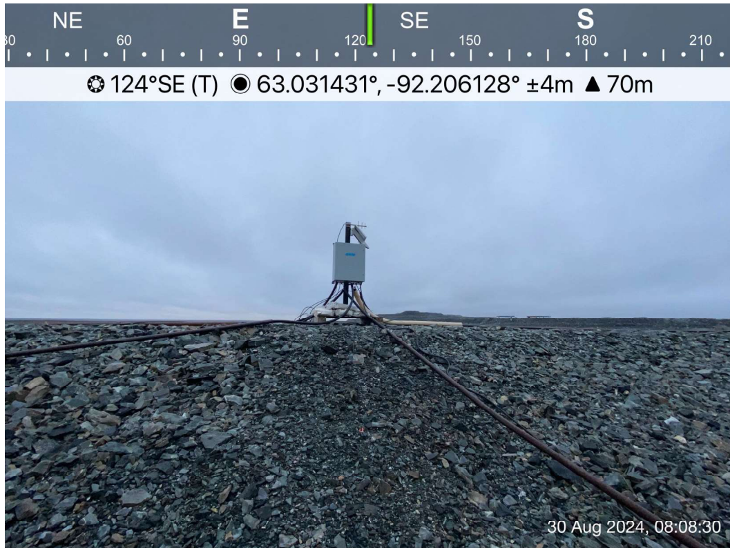
D-CP1 - Photo 5: Dike D-CP1: Ground temperature cable housing and data collection system. Facing southeast.
