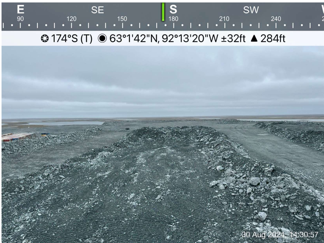
WRSF1 - Photo 4: WRSF1 - Free dumps spread on bench 97 m. Facing south.
