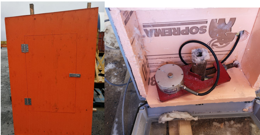
Figure 6. Surface Installation (Shelter & installation inside)
