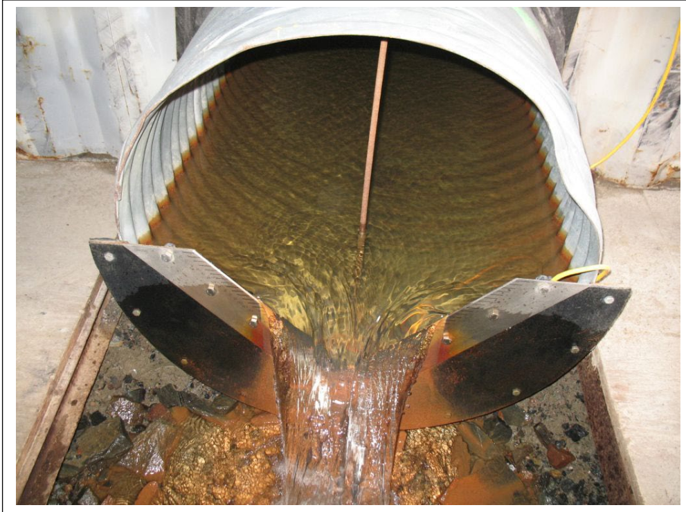
Photo #5 Whale Tail Dike, seepage measuring weir
