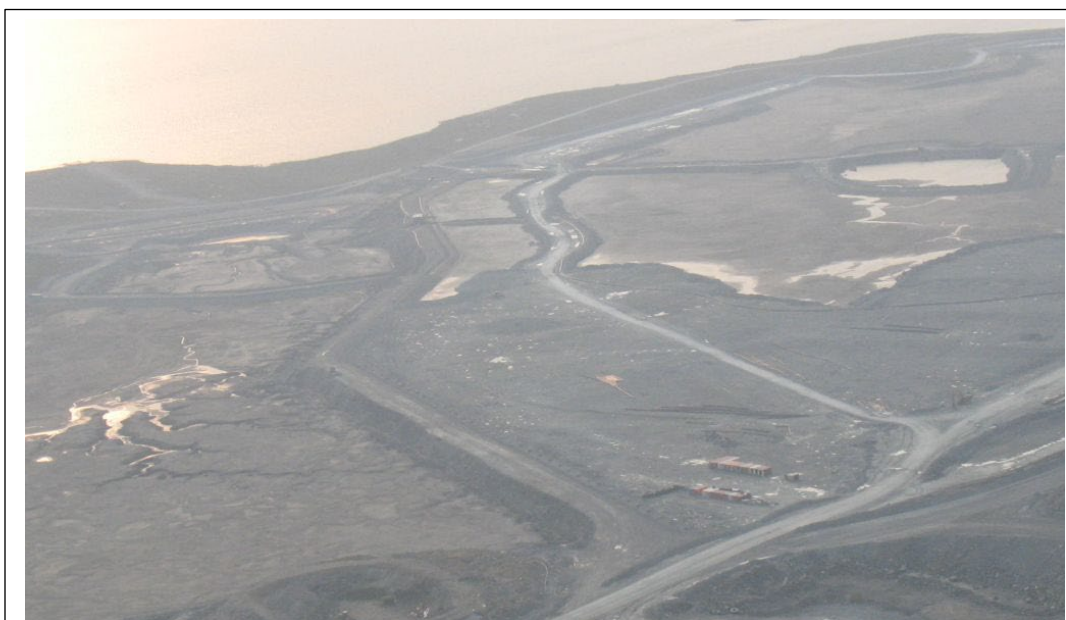
Photo #18 Stormwater Dike and capping of TSF North Cell
