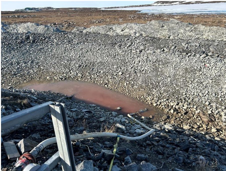
Figure 2. Dyed water from the leaching pad reporting to the mill trench
