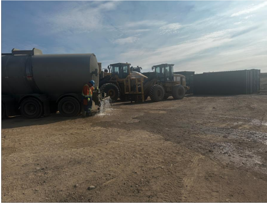
Figure 1 Water truck used to simulate Diesel fuel spill.
