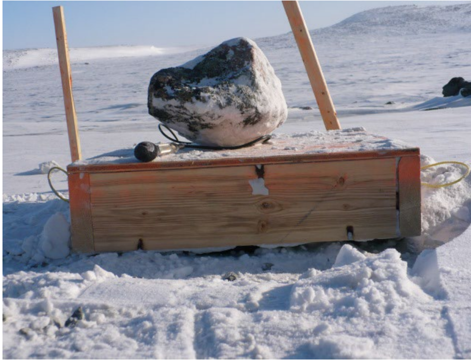
Figure 8: Final Set-up with the microphone in the direction of the blast
