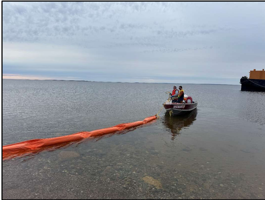
Photograph 7: Boom towing with response vessel and responders.
